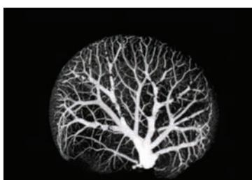
High resolution ex-vivo scan of mouse liver 20 µm voxel size, 35kVp, 1000µA
